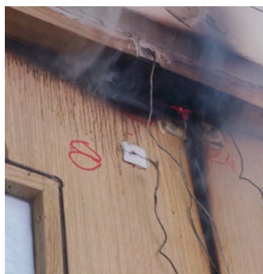
Fire begins to breach door joint
